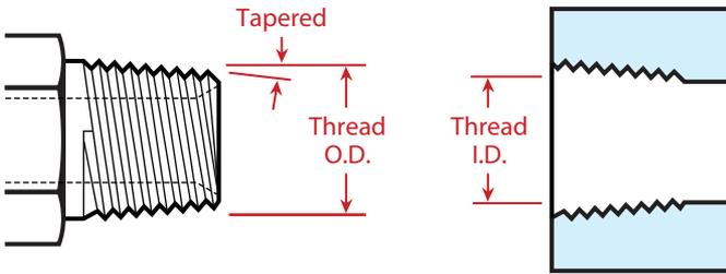
**NPTF Thread Tip:** Measure the thread diameter and subtract one quarter inch to find the nominal pipe size.
